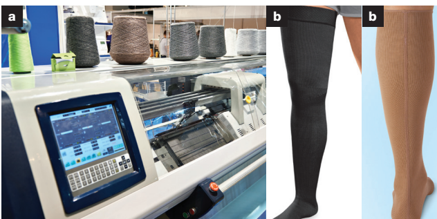
Fig 11. Flat knitting machine (a), examples of flat knit garments (b)
