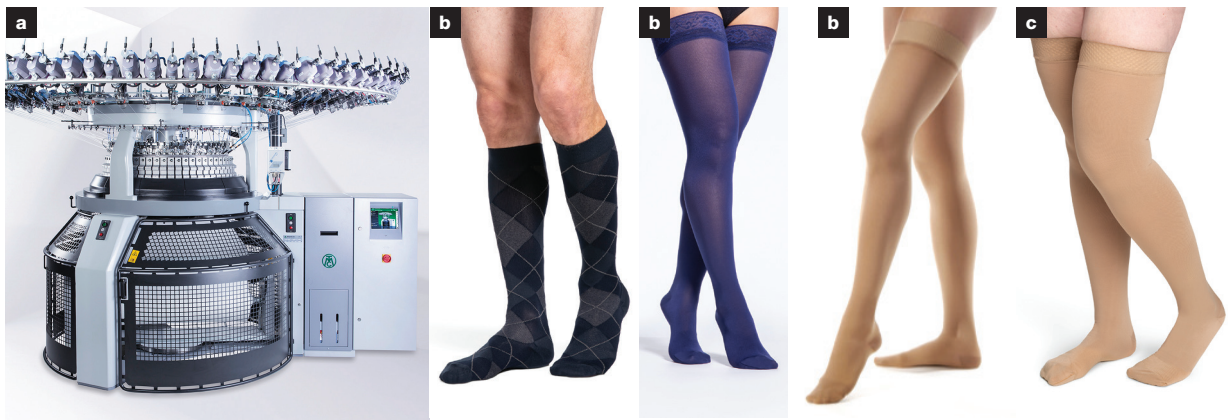
Fig 10. Circular knitting machine (a), examples of circular knit garments (b), example of stiffer circular knit garment (c)
