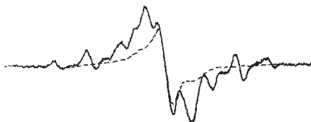
Fig. 2. Electron spin resonance (—) spectra of \gamma -irradiated DNA in vacuum and shortly after introduction of air (---)
