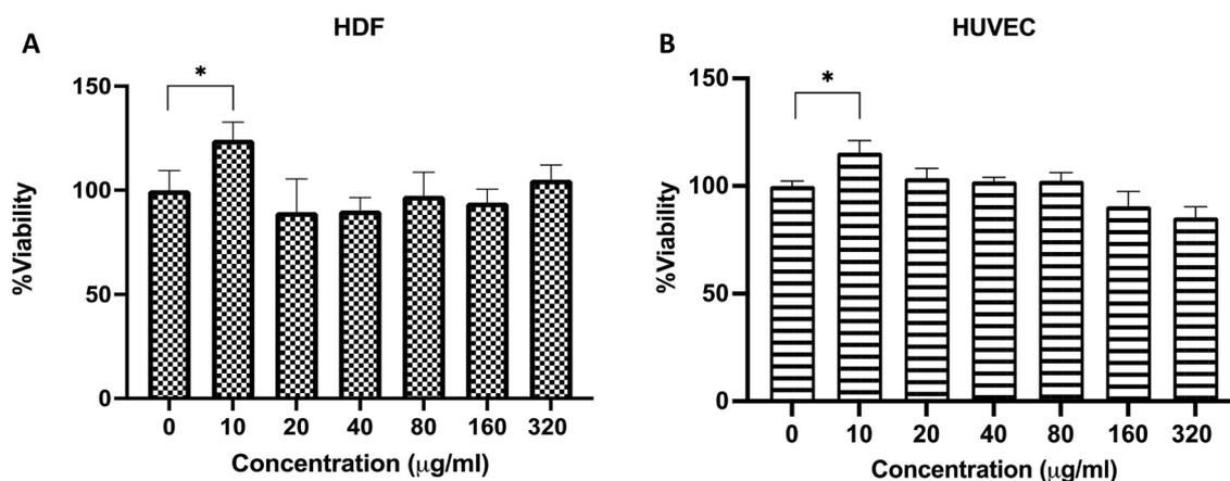
**Figure 1.** Effects of *C. sativus* petal extract on the viability of HDF (A) and HUVEC (B). Cells were seeded in 96-wells plate and allowed to attach for 24 h, then treated with different concentrations of *C. sativus* extract (0–320  $\mu\text{g/ml}$ ) for 24 h. Absorbance was measured at 570 nm using a ELISA plate reader at 570 nm. Results are presented as the means  $\pm$  SEM from three independent experiments performed in triplicates ( $*p < 0.05$ ).
